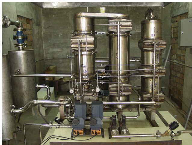
Fig. 2. Photograph of 75-kw methanol auto-thermal reforming fuel processor.
